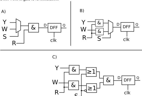
Circuit A shows a D-flipflop that is synchronously reset to zero by a reset input signal R. When it is not reset, it is fed by a multiplexer with inputs Y,W,S that we assume are unknown and therefore X during reset. The implementation in circuit A is guaranteed to correctly reset the flip flop in simulation since the AND cell simulation model will see one of its inputs as zero and therefore know the output must become zero even if the output of the multiplexer is X.
