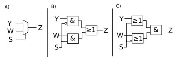
This example consists of a two-to-one multiplexer that forwards either its Y or W input depending on the value of S. Three variants are shown, A) using a monolithic multiplexer cell, B) implemented with and-or logic, C) implemented with or-and logic. All the three variants of the multiplexer shown have the exact same truth table, as shown below, and the synthesis tool is allowed to generate any of them.
